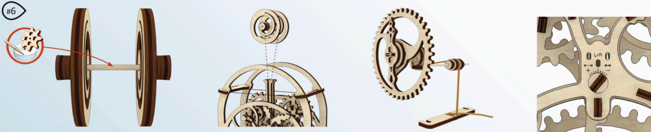
**5** **ENG** If the pendulum and roller continue to operate erratically after preforming all of the above troubleshooting steps: Take the pendulum out of the Timer, remove all three axles from the pendulum, and replace the axles with new one. Be sure the new axles is straight and that all parts are properly aligned. Use solid candlewax to lubricate the pendulum axles. (Figure 7)
