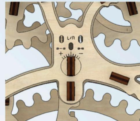
**4** **ENG** Use solid candlewax to lubricate the roller axle and replace the roller in the pendulum. Check the Timer against a standard clock. Adjust the tension in the rubber band. If the timer still does not run continuously, increase the tension in the rubber band. If the Timer begins to operate erratically, decrease the tension in the rubber band. (figure 6)
